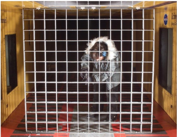
Figure 2.—A technician measures the thickness of ice accreted on the Grid.
