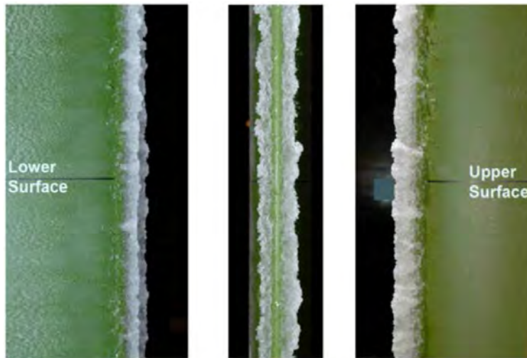
Fig. 14 Experimental ice accretion photographs for case 242, run ED1978*.
